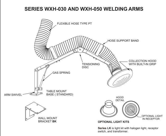
Note: 3 foot standard arm supplied with 5 feet of hose, 5 foot arm supplied with 7 feet of hose.
