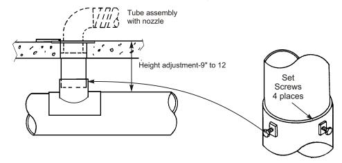
4. Place and level saddle completely over the opening. If underfloor duct size is slightly larger than the saddle size, pressure can be applied to "open" the saddle to conform to the transite diameter.
