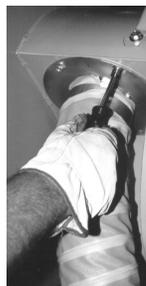
Make sure gasket is in place between tube and reel flange
