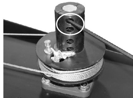
Loosen bolts on clamping collar to rotate drum on reel. After adjustment is made, all 8 bolts must be tightened to 14.5 lbs of torque.
