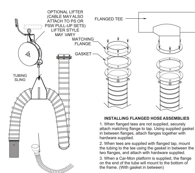
NOTE: In some instances, a tubing sling is not used. The lifter cable may be attached directly on the adapter or to a cable and clamp directly behind the adapter.
