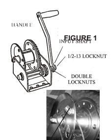
\_Thread cable through hole in side of drum
