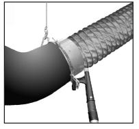
The positioning pole pull-down knob is inserted in the hole in the lifting ring on the EPDM adapter. The adapter is usually attached to the cable from the retractor or balancer. Pull the adapter assembly down far enough to fit over the exhaust pipe. After use, pull down the adapter enough to dis-engage the retraction of the retractor or balancer unit. Check operation instructions that were provided with
