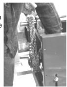
Loosen bolts on motor base to put tension on the belts, one side at a time, checking after each side to make sure the moror drive is leve with the fan wheel shaft.
