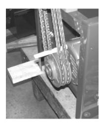
Check level of motor pulleys and shaft to make sure they are the same.
