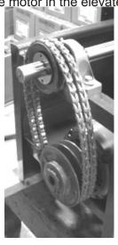
When tension is off belts, they can be removed from pulleys.
