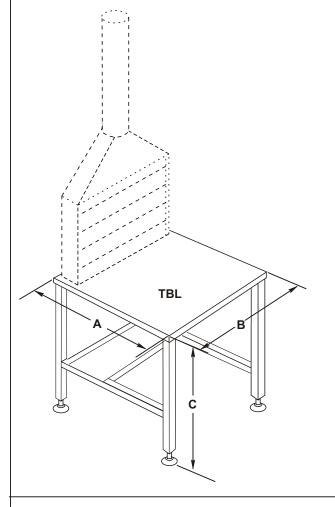
Series TBL welding tables are 32" high, and include top plate, tubular steel frame with shelf, and leveling feet with  $\pm$  3" height adjustment.
