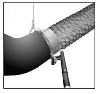
The positioning pole pull-down knob is inserted in the hole in the lifting ring on the EPDM adapter. The adapter is usually attached to the cable from the retractor or balancer. Pull the adapter assembly down far enough to fit over the exhaust pipe. After use, pull down the adapter enough to dis-engage the retraction of the retractor or balancer unit. Check operation instructions that were provided with the retractor mechanism.
