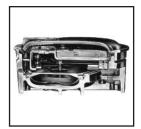
in response to the position of the magnet without mechanical linkages. Cutaway view of the Magnehelic® gage showing the actuating diaphragm, the leaf spring with magnet, the helix which turns the indicating pointer
