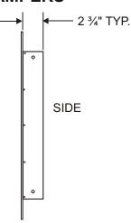
NOTE: Car-Mon Automatic Closing Back Draft Dampers feature heavy gauge extruded aluminum construction with aluminum damper blades, nylon bearings and felt pad seal. When ordering, indicate quantity and size of fan for which damper is required.
