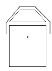
NOTE: Car-Mon Weather Covers are constructed of formed 18 ga. cold-rolled steel, polyester powder coated. Features include clipped corners for safety and slots for attachment with  $\frac{1}{4}$ -20 hex bolts.
