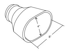
Series **ROW** adapter is specially constructed with a wider opening to accommodate side by side dual exhaust configurations. For use with 3" or 4" hose.
