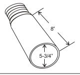
Series **RS** adapter is an EPDM adapter for use on cars and trucks. For 4", 5", or 6" hose.
