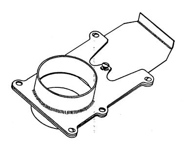
Car-Mon Series BG Blast Gate Dampers are of 2-piece cast construction with fully adjustable sliding gate and set screw for permanent damper setting. Applications include use on duct for dust collecting systems and on carbon monoxide or welding fume exhaust systems. Other sizes available on request.
