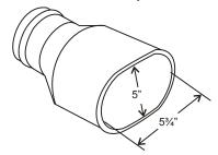
Series **RO** is a versatile adapter designed for use on cars and small trucks. For 3" or 4" hose
