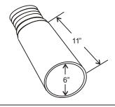
Series **RS** adapter is a straight type adapter for use on cars and trucks. For 4", 5", or 6" hose.
