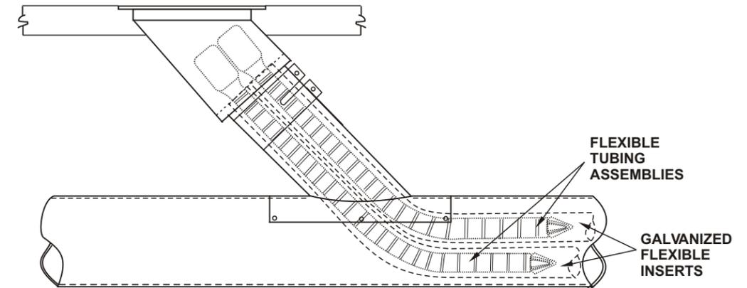
When installing dual units, the galvanized flexible insert assembly must be placed in unit prior to installing tube assemblies. Insert assembly will remain in place, and tubes will slide in and out of the insert.
