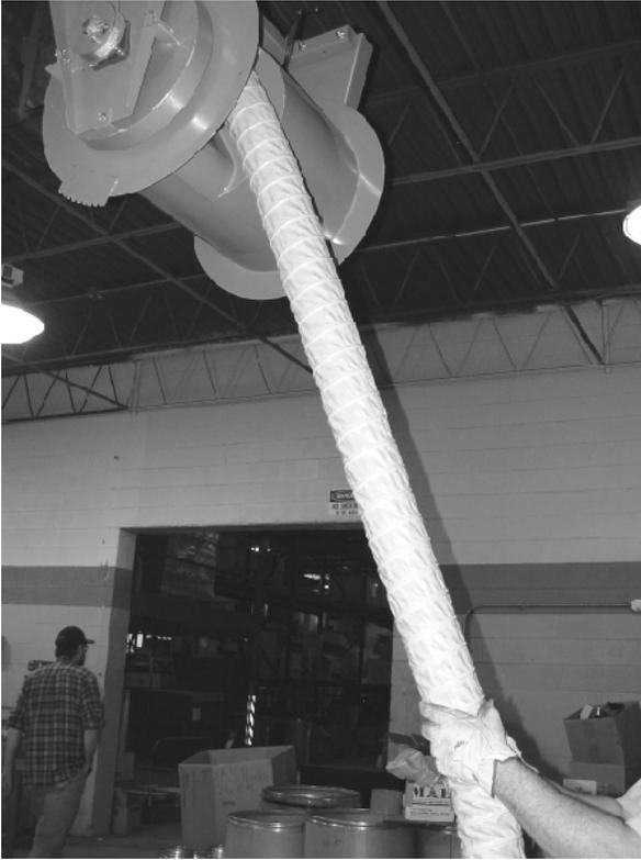
**VERY IMPORTANT!** When retracting the tubing grasp the tubing and guide it up onto the reel, making sure that the tubing does not overlap. After the tube starts to make the last wrap on the reel, let go of the tubing
