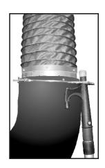
After pulling the hose assembly down, insert the positioning part of the pole into the hole on the lifting ring as shown on left, and position the adapter over the diesel stack as shown on right.
