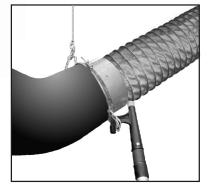
The positioning pole pull-down knob is inserted in the hole in the lifting ring on the EPDM adapter. The adapter is usually attached to the cable from the retractor or balancer. Pull the adapter assembly down far enough to fit over the exhaust pipe. After use, pull down the adapter enough to dis-engage the retraction of the retractor or balancer unit. Check operation instructions that were provided with the retractor mechanism.
