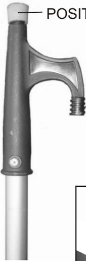
POSITIONING KNOB: Used for positioning the adapter on to the exhaust pipe.
