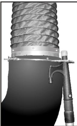
After pulling the hose assembly down, insert the positioning part of the pole into the hole on the lifting ring as shown on left, and position the adapter over the diesel stack as shown on right.
