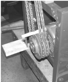
Check level of motor pulleys and shaft to make sure they are the same. Make sure the pulleys are aligned properly. Allow for bushing to draw sheave when tightening. After adjustment "peen" key in bushing with punch.
