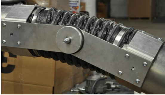
Illustration F: WXS Arm Back & Middle joint assembly; to tighten or loosen use a 9/16 wrench.
