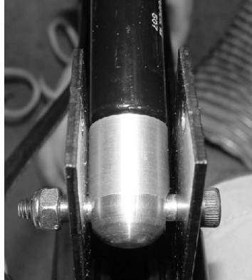
Gas Spring bottom attachment detail
