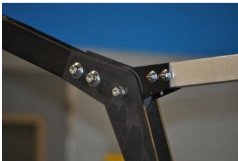
Illustration B: L Bracket Connection to Support structure; place (2) 3/8-16 x 2.25” bolts thru matching holes secure and tighten with 3/8-16 Whiz-lock nuts
