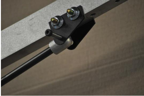
Illustration D: Shoulder bolt placed thru holes in bracket; secured with nylock nut. Use 5/32 Allen wrench to hold shoulder bolt in place while tightening with 3/8 wrench
