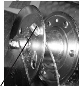
Thread cable through hole in side of drum
